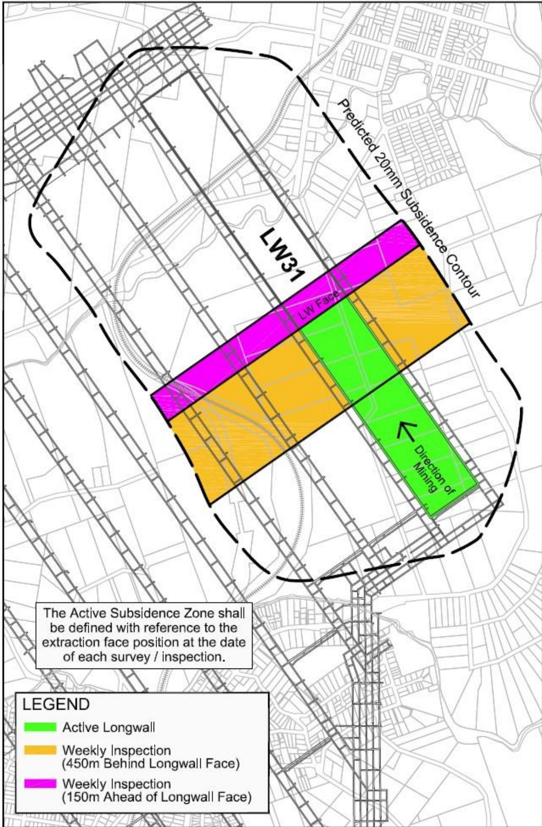
Figure 2 Diagrammatic representation of 'active subsidence zone'
