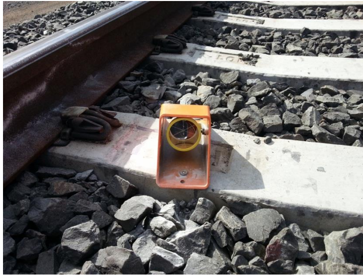
Fig. 2.5 Typical survey prism on railway sleeper
