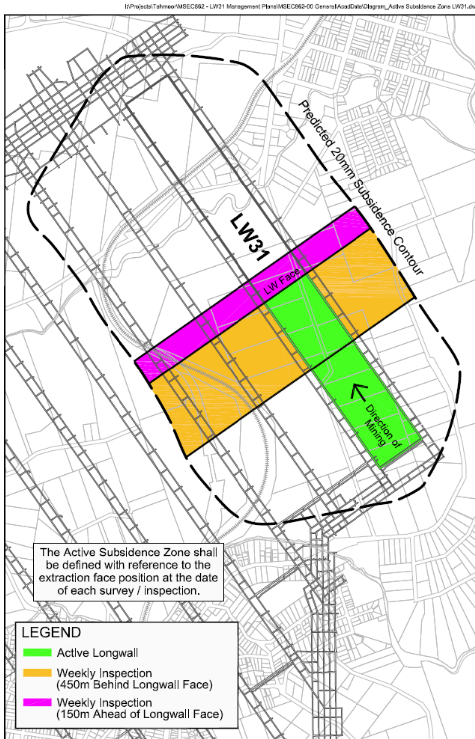
Fig. 1.1 Diagrammatic Representation of Active Subsidence Zone
