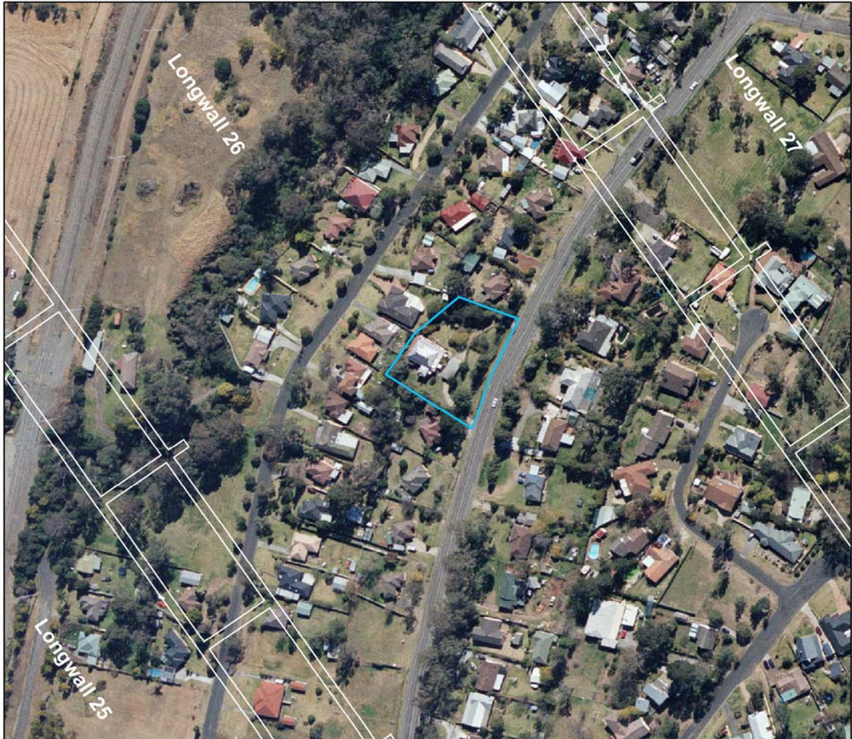
Fig. 1.2 Location of No. 55-59 Remembrance Drive, Tahmoor in relation to Tahmoor Longwall 26
