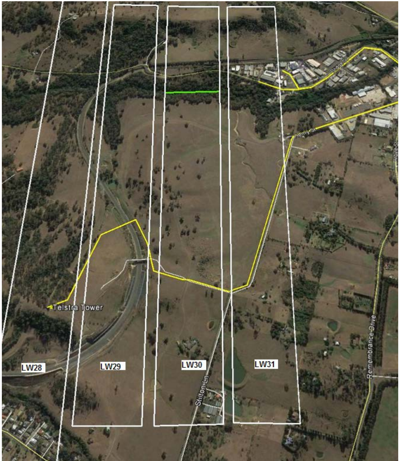
Plate 1: Google Earth aerial view of four longwalls LW28 to LW31 showing current location of extraction in LW30 (Green Line). Longwall LW31 extends north-west from north of Remembrance Drive at Tahmoor, crosses Stilton Lane and then Bridge Street and the Main Southern Railway in the north to the west of Picton. The yellow lines indicate Telstra optical fibre cables, two sections of cable F PCTN 3002 A) and B) feeding along Bridge Street and south section along Stilton Lane to the Telstra Tower
